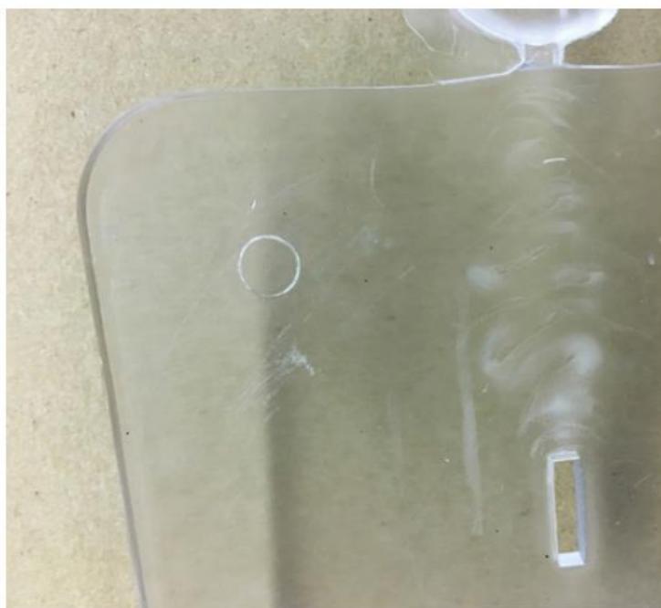
Figure 21.2 Jetting in a clear polycarbonate plaque resulting in a cloudy appearance
