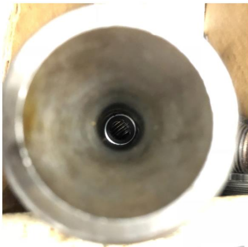
Figure 21.3 Hang up step (shiny inner diameter) looking through the end of a nozzle towards the tip
