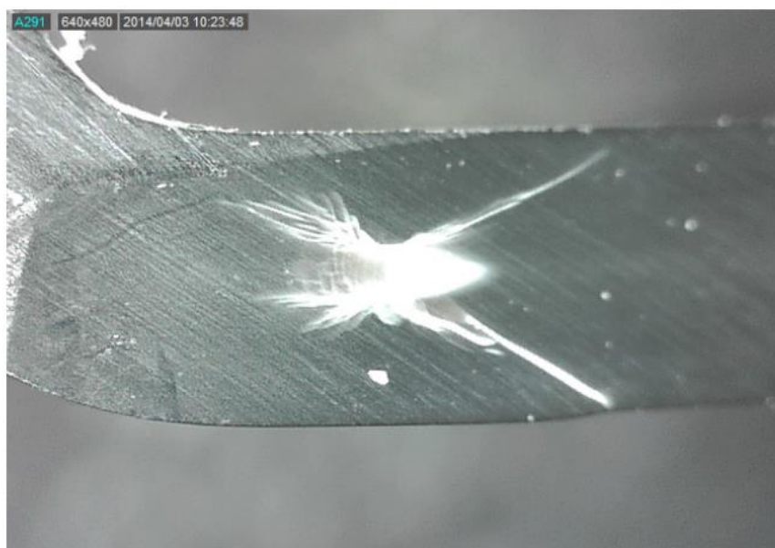
Figure 23.10 Single-pellet contaminant in wall stock
