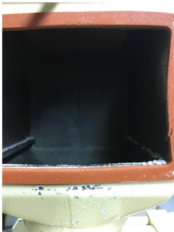
Figure 23.2 Pellets stuck in magnet drawer
