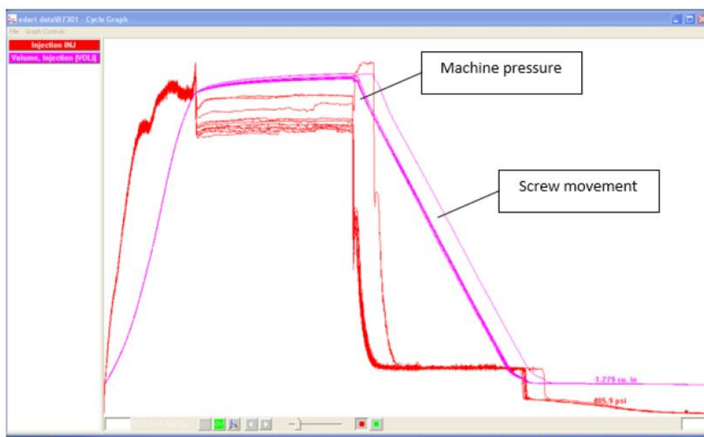
Figure 26.7 RJG eDART® showing 10 consecutive shots with second-stage pressure variation
