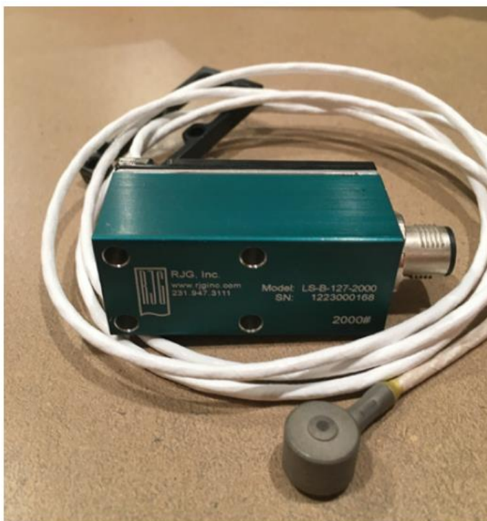
Figure 26.1 RJG cavity pressure transducer
