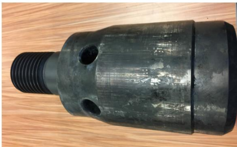
Figure 26.6 Ball check non-return valve
