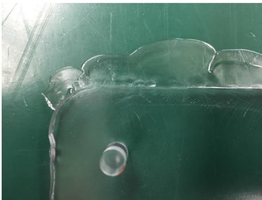
Figure 30.3 Part flashed from transferring too late
